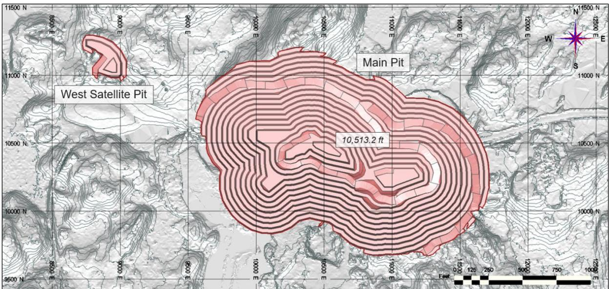
Figure 16-20: Crean Hill Waste Rock Dumps and End-of Open Pit Mining
