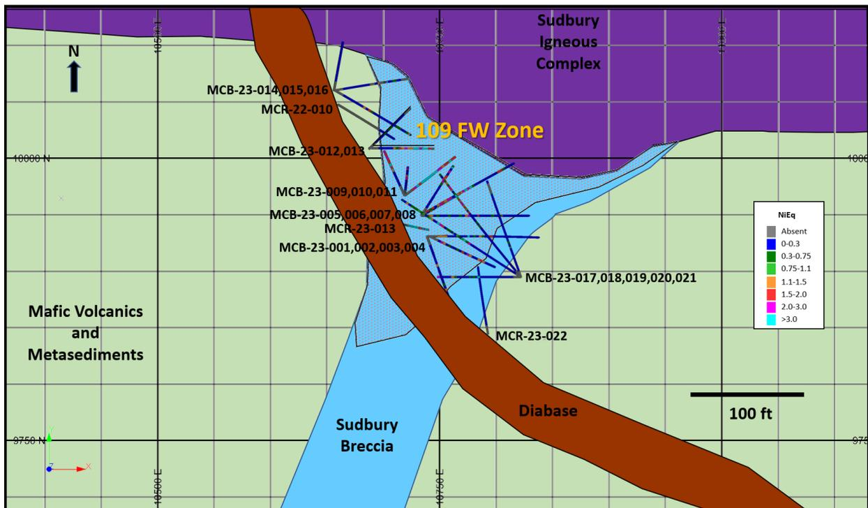
**Figure 10-5: Longitudinal Section of the Crean Hill 101 Footwall Zone. Magna Diamond Drillholes and the Location of Section B (Figure 2) are Illustrated. Refer to Figure 10-3 for the Location of Longitudinal Section A-A' (Source – Magna Mining)**
