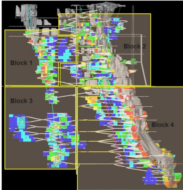
Block 1 and Block 3 are primarily greenfield production areas with longitudinal longhole as the primary mining method. Block 2 and Block 4 are brownfield production areas with cut and fill used near historic workings and longhole used in areas not influenced by previous mining.
