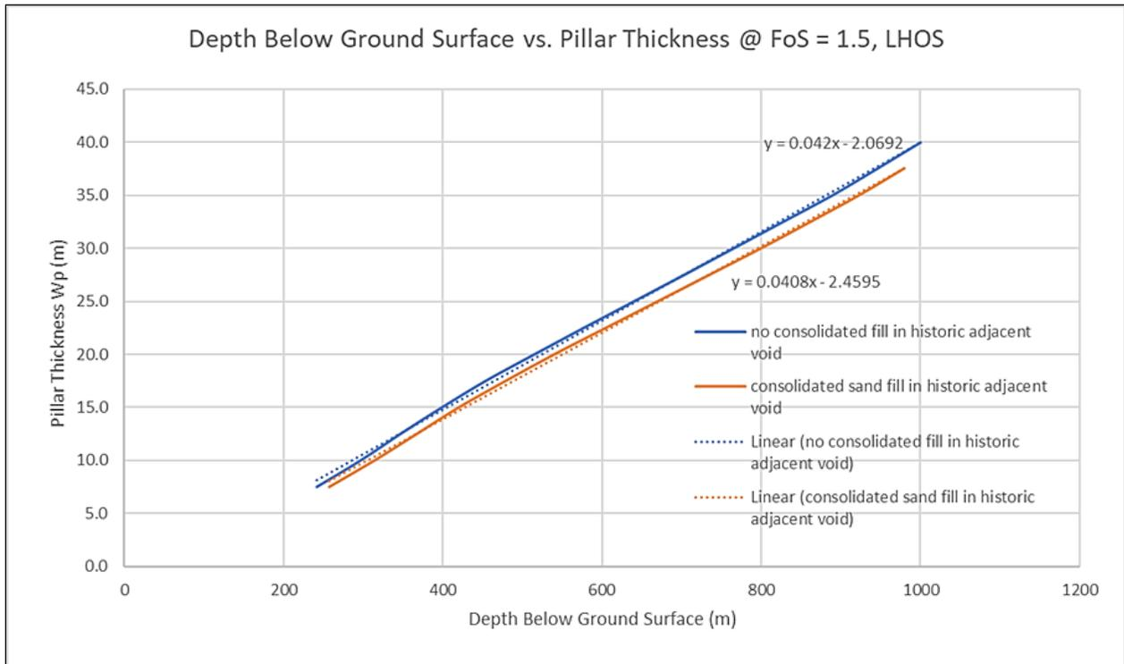
The pillar thickness required for cut and fill stopes near historic mined out areas at a factor of safety of 1.5 is demonstrated in Figure 16-26.
