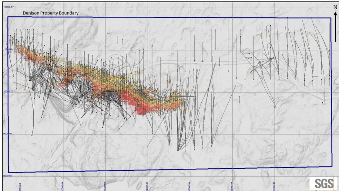
**Figure 14-2: Isometric View Looking North – Distribution of Surface and Underground Drill Holes on the Crean Hill Property in Local Mine Grid**
