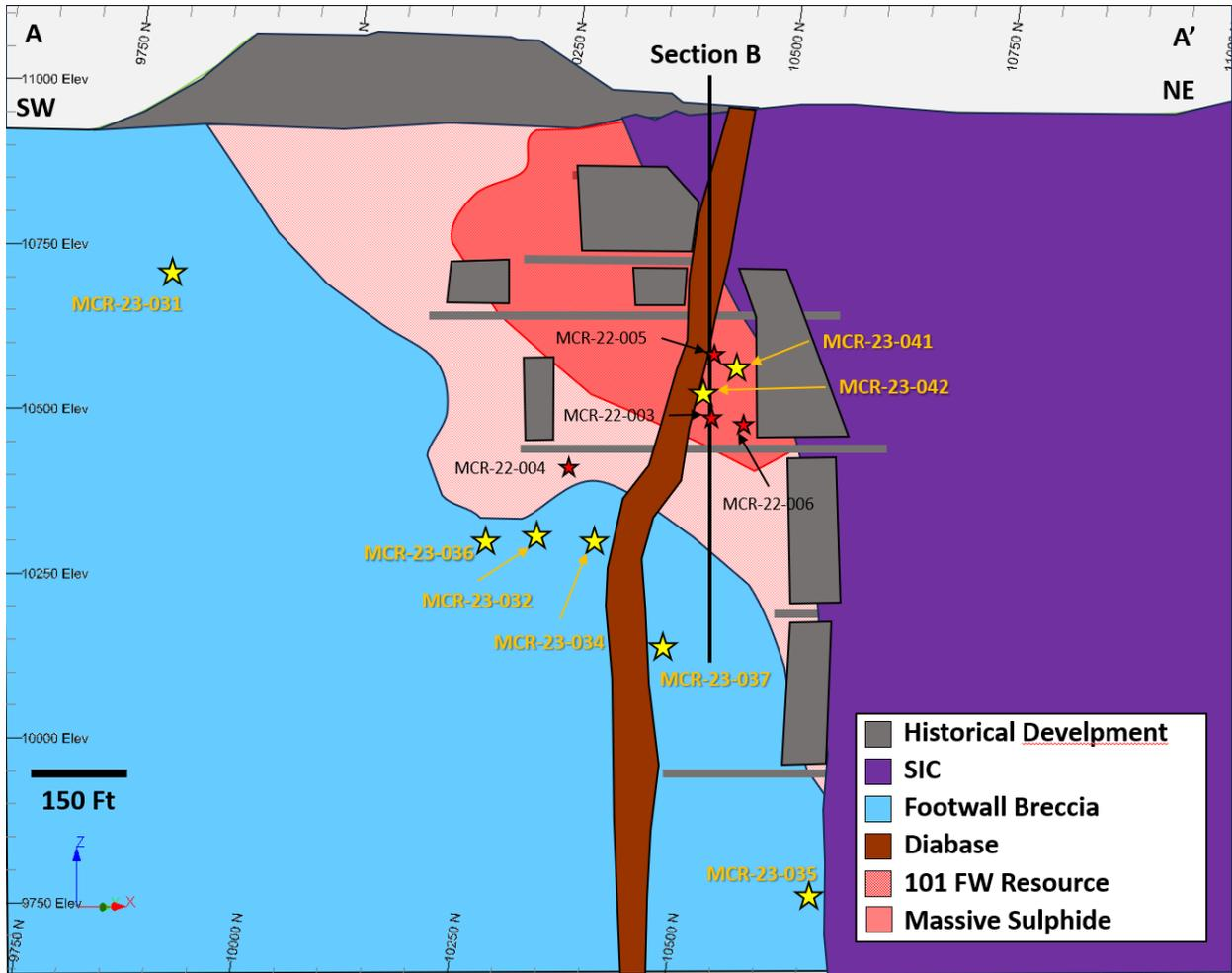
**Figure 10-6: Vertical Section B, through the 101 FW Zone, Showing General Geology, Recent and Historical Drilling Results, and the Current Resource Model. Refer to Figure 10-5 for location of Section B (Source – Magna Mining)**
