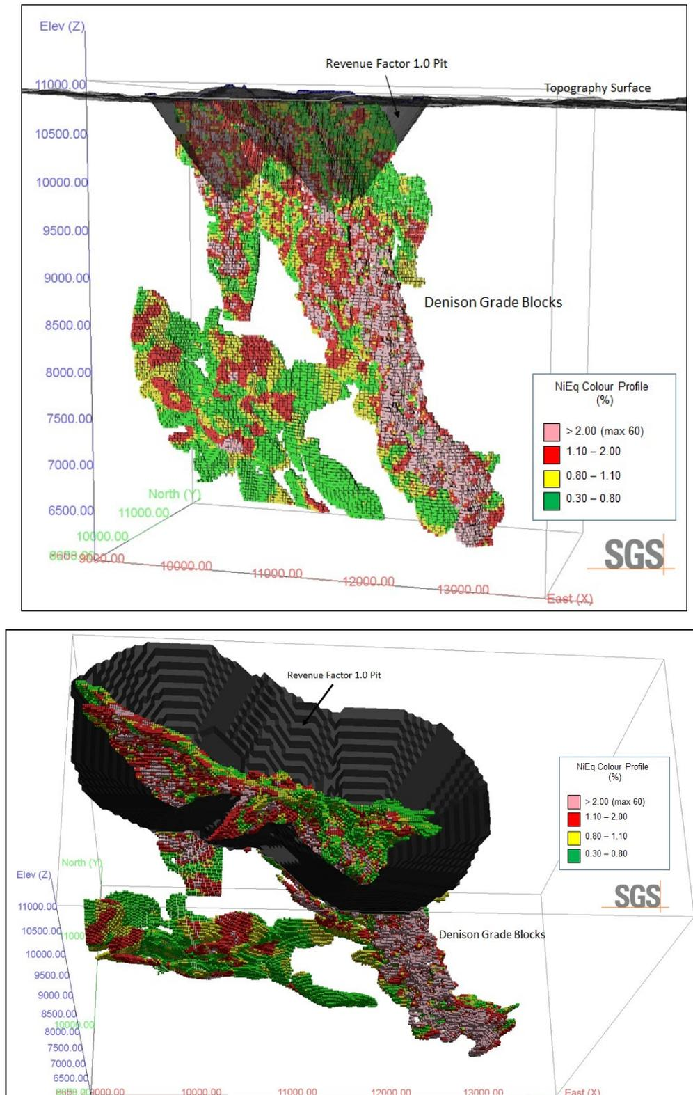
**Figure 14-9: Isometric View Looking North of the Crean Hill Deposit Indicated and Inferred Mineral Class Blocks and Whittle Pit (upper and lower image)**
