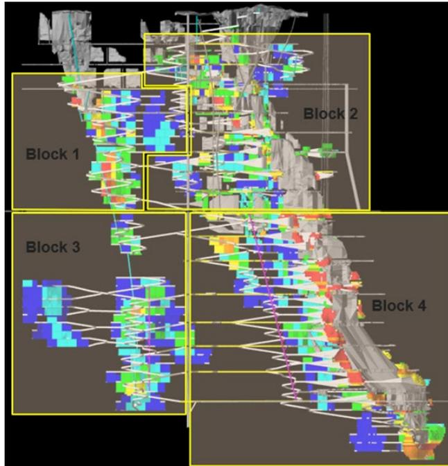
Block 1 and Block 3 are primarily greenfield production areas with Longhole as the primary mining method. Block 2 and Block 4 are brownfield production areas with MCAF used near historic workings and Longhole used in areas not influenced by previous mining. Sublevels will be spaced at 82ft (25 m) vertical intervals, with some variation to accommodate existing development.
