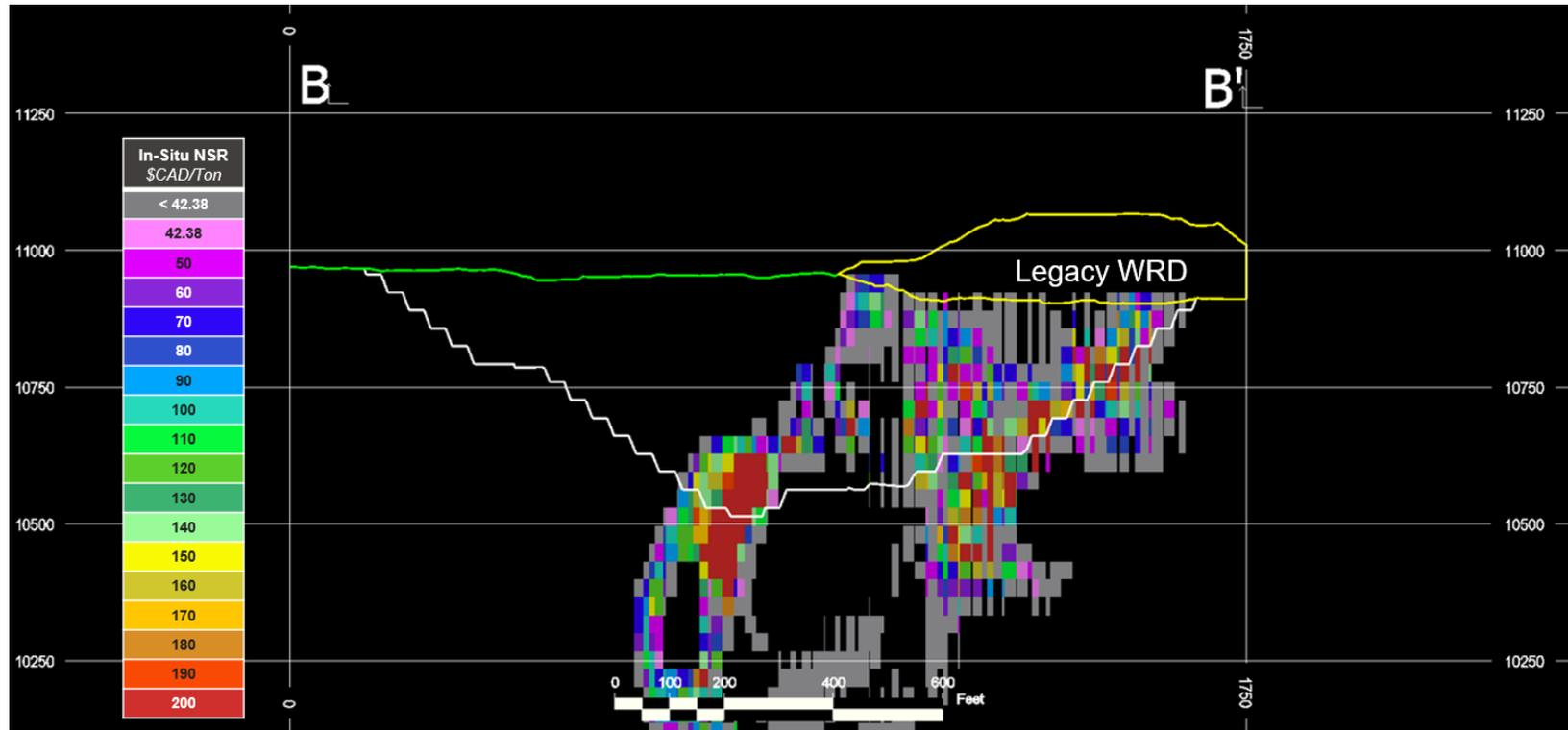
Figure 16-8: Cross section CC' through the east lobe of the main pit
