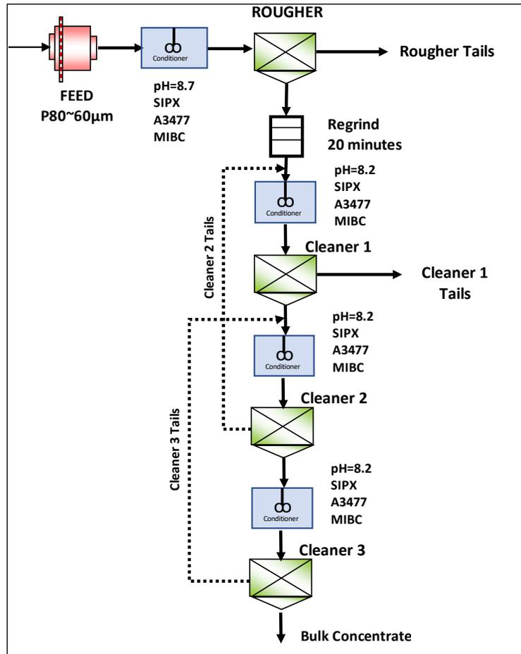
A LCT is used to simulate the conditions of a plant where internal streams are circulated. There were two LCTs performed, each containing six cycles; stability was achieved in both tests (refer to Figure 13-6).
