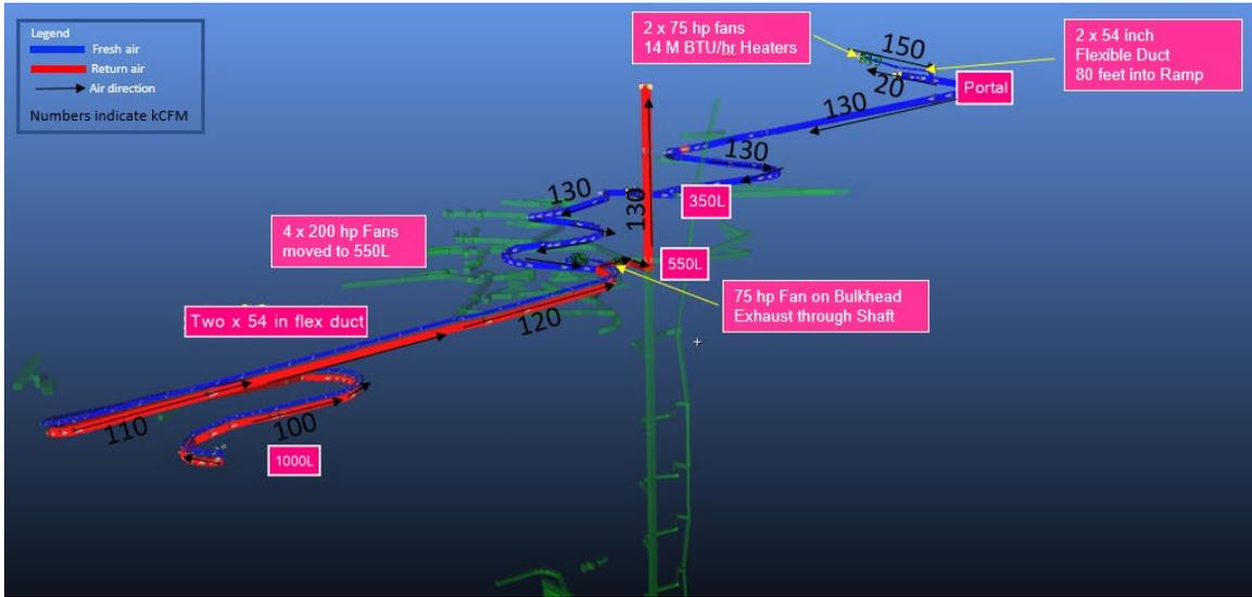
Once development reaches 1000L the Access Ramp will connect to existing development to allow the ventilation loop to be advanced to 1000L. Booster fans will be installed on 1000L to increase ventilation flows to 300 kcfm to allow increased underground activity. The shaft will continue to be used for exhaust air. The ventilation configuration once the Access Ramp reaches 1000L is shown in Figure 16-41.
