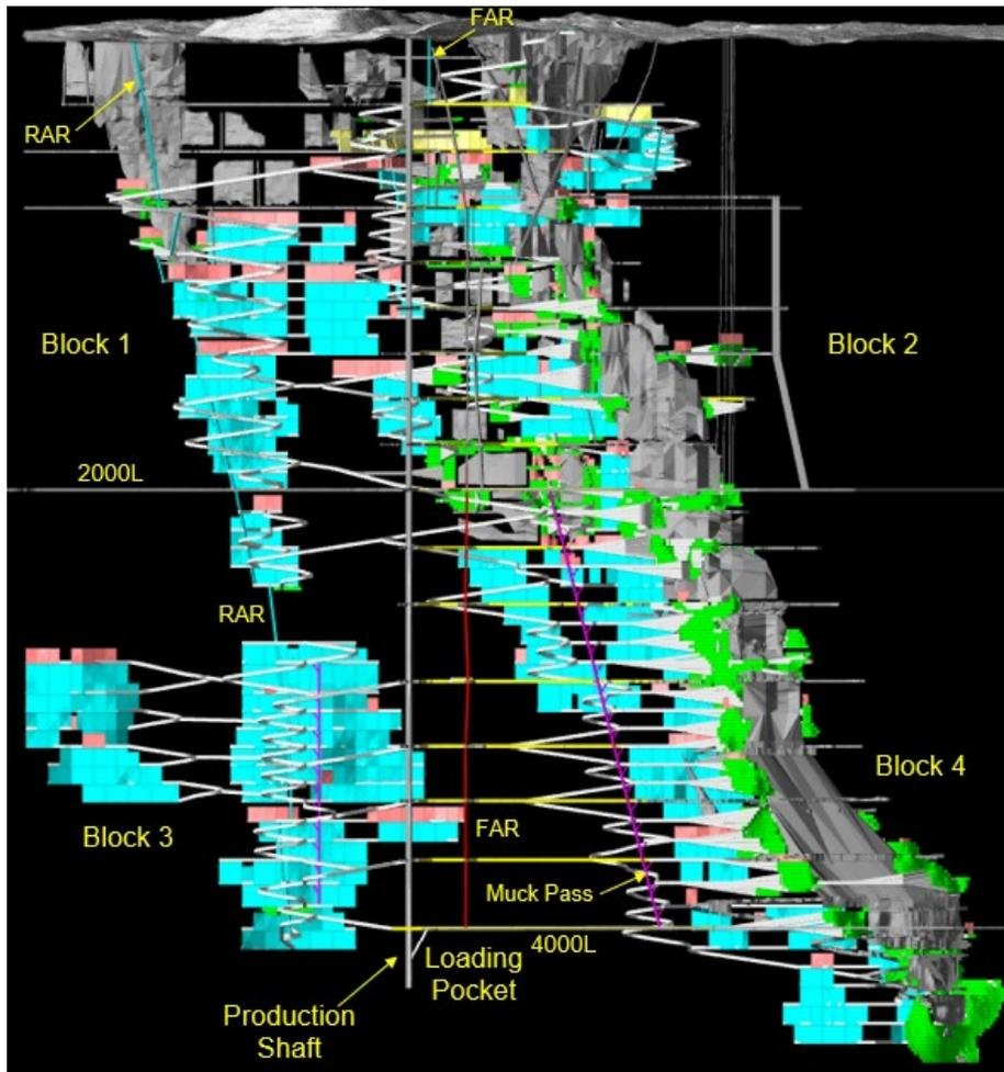
The final combined Open Pit and Underground Mine Design at the end of the mine life is shown in an isometric view in Figure 16-36.
