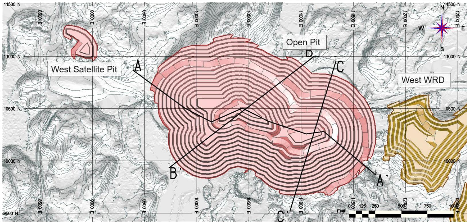
The pit is shown with 16.4 ft (5 m) contours, topography is shown with 5 ft (1.5 m), and the west waste rock dump (WRD) is shown with 8.4 ft (2.5 m) contours.
