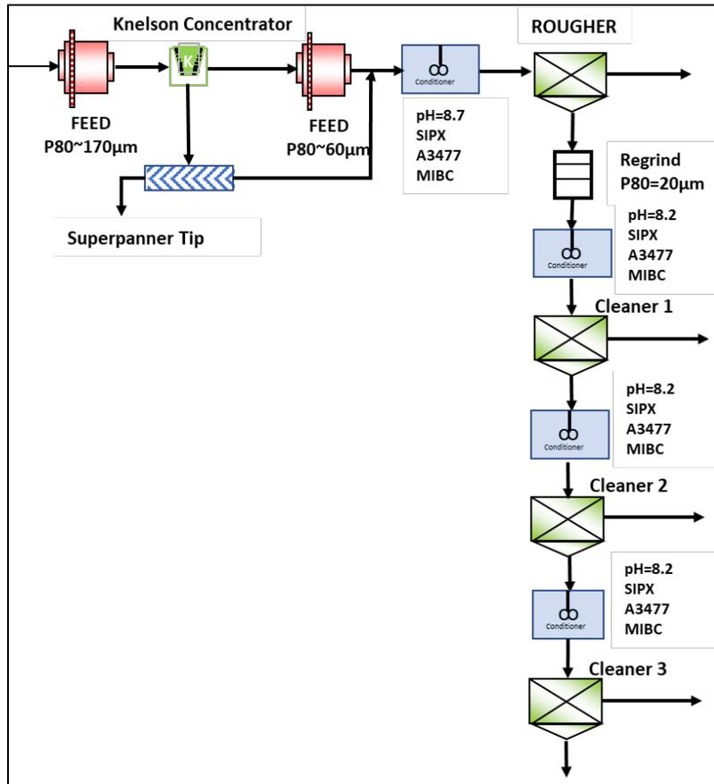
**Figure 13-10: Open Circuit Gravity/Flotation Test Results (Source: XPS, 2023)**
