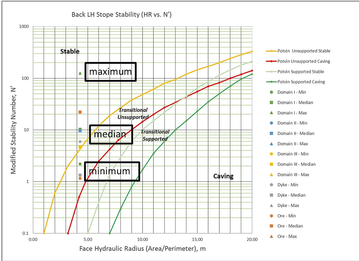
**Figure 16-24: Slope Stability – Slope Hangingwall/Footwall**
