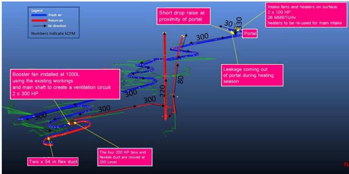
The final ventilation configuration for Phase 1 will include a new 13-ft diameter return air raise (RAR) to surface and a short 16.4-ft diameter fresh air raise (FAR) near the shaft to provide 812 kcfm. The new FAR will connect to the shaft through lateral workings on 350L and the shaft will become the fresh air intake. An existing raise that parallels the shaft will also be used for fresh air intake. The final Phase 1 ventilation configuration is anticipated to include the following.
