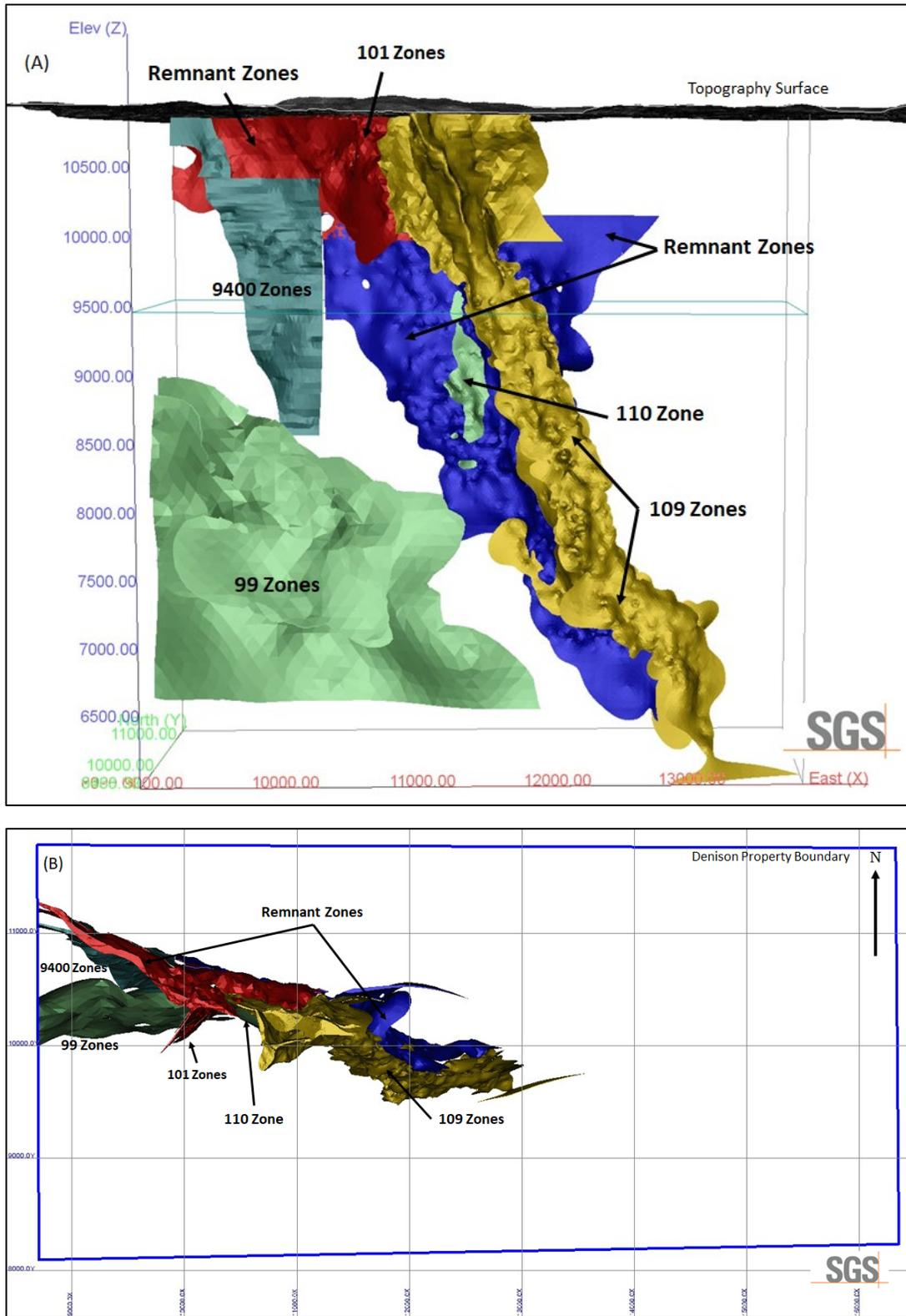
**Figure 14-4: Crean Hill Diabase Models – Isometric View Looking North**
