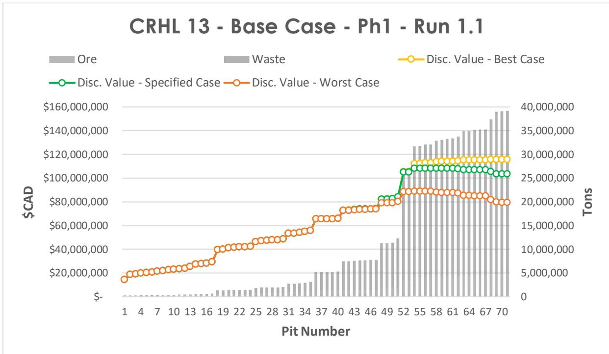
For the second stage of the pit optimization, pit 48 above was used as the topography. The software was re-run and another set of optimization results were obtained.
