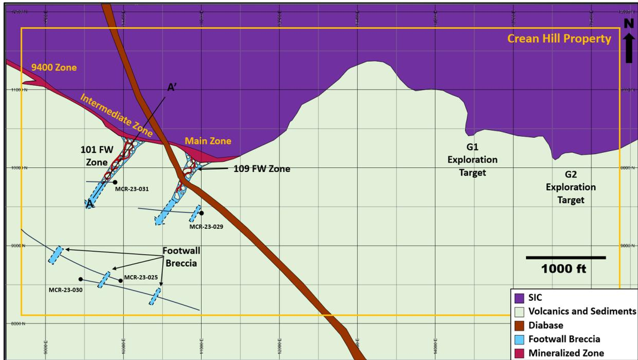
Figure 10-4: Plan View of the 109 FW Zone, Showing the Location of Near Surface Drillholes (Source – Magna Mining)
