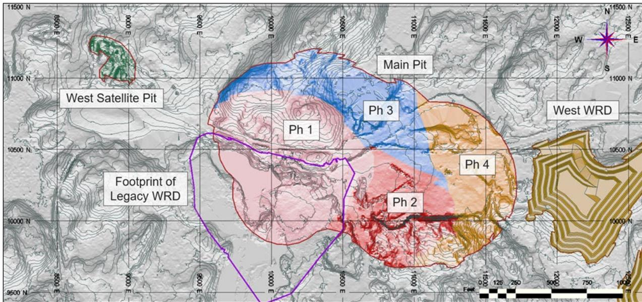
Phase 1 was designed to be the starter pit because it contains material accessible at a relatively low-strip ratio. Phase 2 was designed to primarily be a waste stripping pit that can be mined while Phase 1 is developed. Phases 3 and 4 are much larger and require an advance pre-stripping effort to support sustained production.
